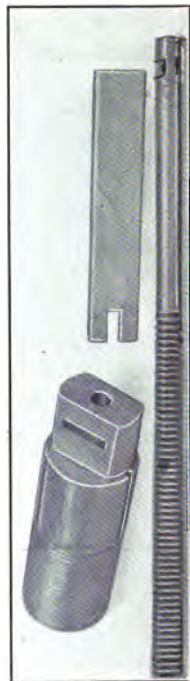
FIG. 39B.—Broach, holder and cutter.
